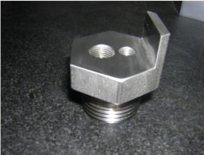
*Illustration- If you look closely at this part, you'll notice chamfered edges, the tops of holes deburred with a light countersink, and machined surfaces lightly buffed to improve the appearance. These are typical "standard practice" finishing details often added by machine shops. Note that none of these features are on the part print. If you want something done differently (a sharp edge, for example), be sure to call it out on the print.*
