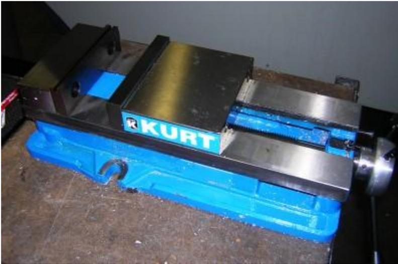
*Illustration- A Kurt-style vise is the most common workholding device in the shop. The most common of these vises have 6" long jaws which open about 9".*
