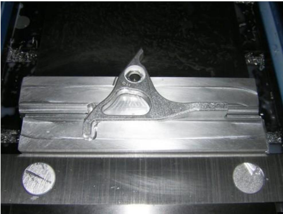
*Illustration- Machined aluminum softjaws, like these in a 6" Kurt double vise, are a common way to*
